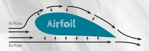
Because of the curved shape of the top of the wing, the air flowing over the top has greater distance to travel and moves faster, which reduces air pressure.
